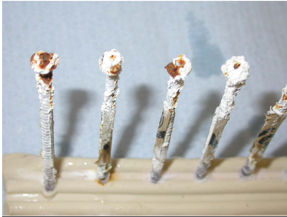
The photograph showing the condition of the Timco Firmahold Collated Nail Samples after 168 hours Salt Spray Test
